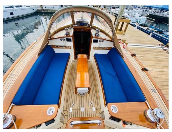
The two secondary winches on the house top provide push button control of centerboard pennant, spinnaker halyard, main halyard and preventer. All lines have flush, stainless steel lined bins for clutter-free storage. All four deck winches are stainless steel *Lewmar* two-speed electric.
