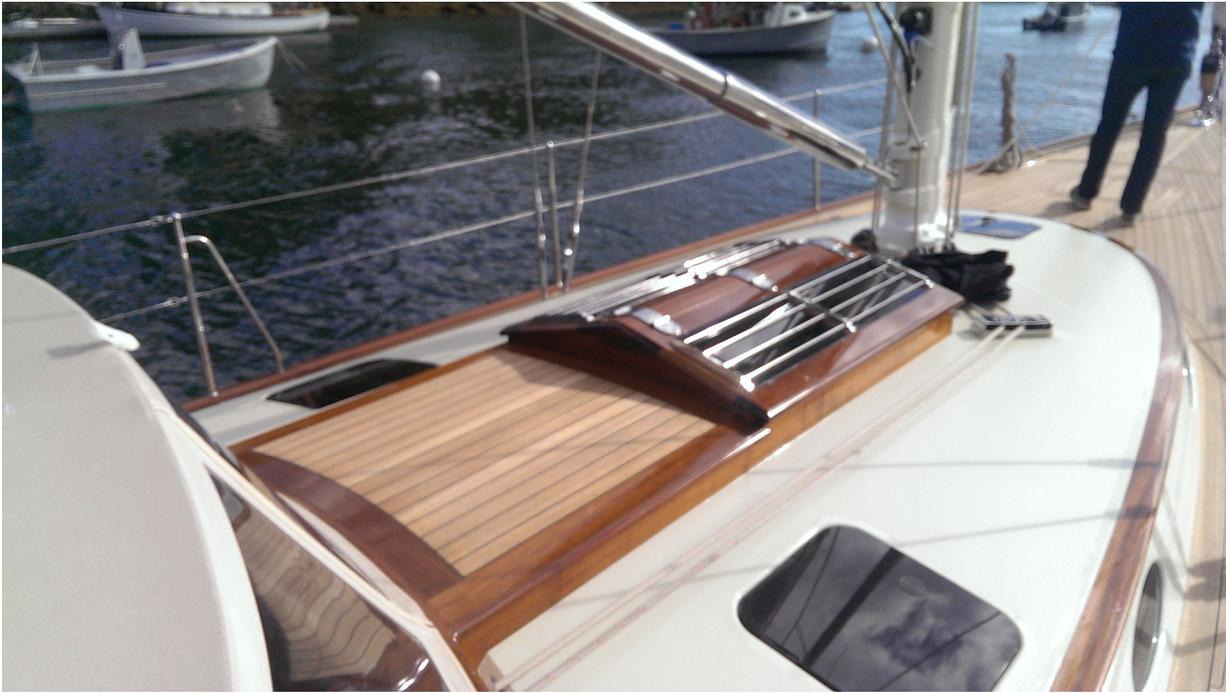
Custom teak and stainless-steel opening skylight and flush opening deck hatches.
