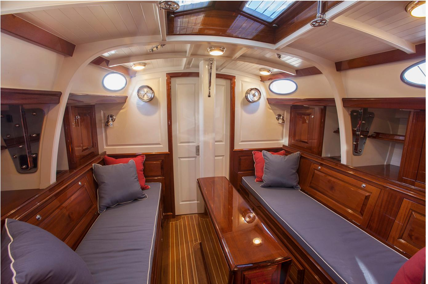
Raised panel sliding pocket doors slide to create an open and full access to the forward cabin.
