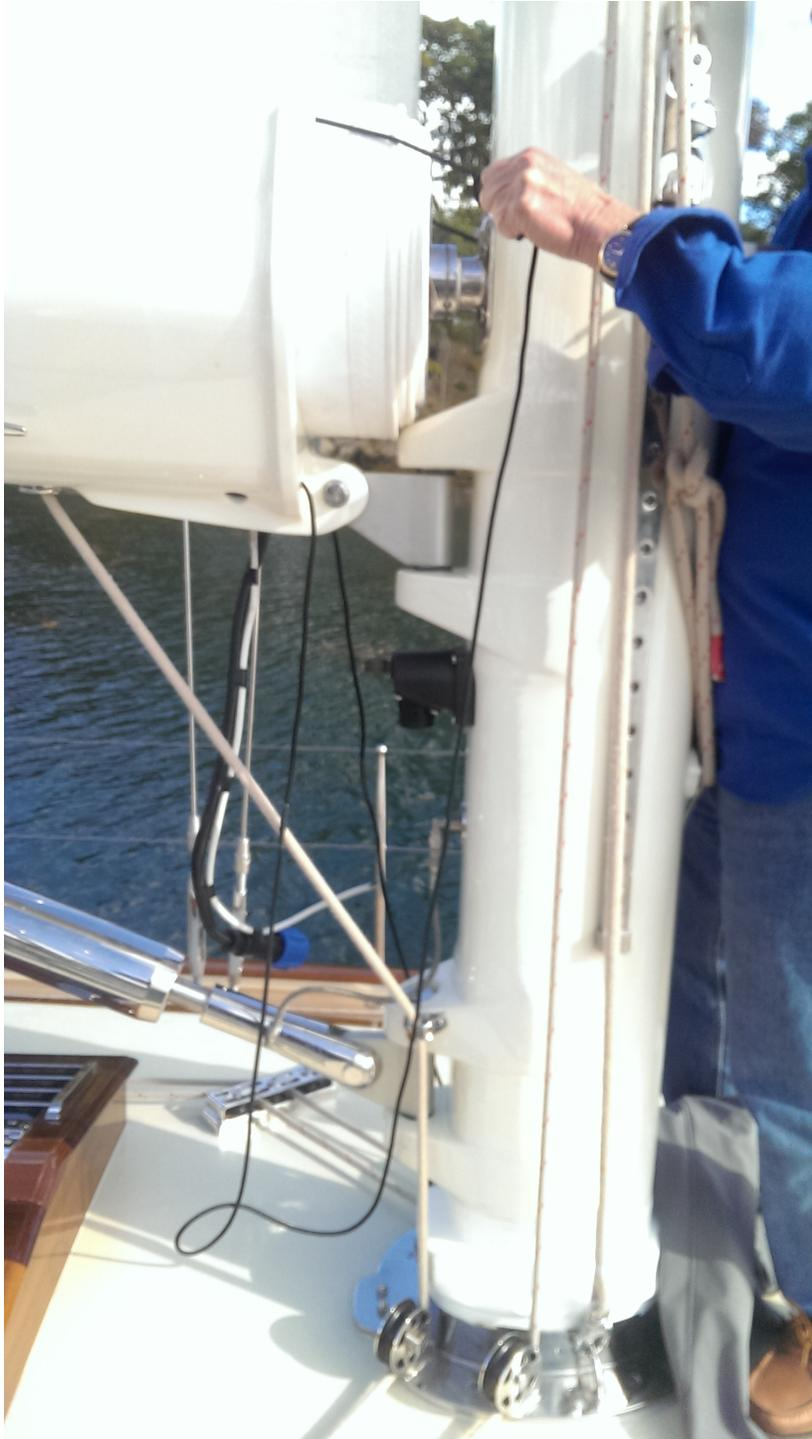
Carbon fiber mast with hydraulic carbon in boom furling system. Stainless steel hydraulic vang, hydraulic in-boom main furler, and mast collar with custom built-in stainless steel turning blocks.
