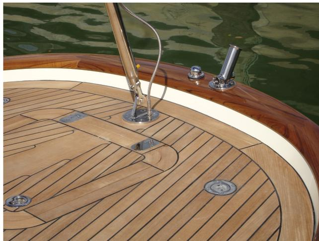
Aft deck – huge lazarette for storing fenders and dock lines, custom flag socket with bracket for propane grill, stainless steel hydraulic backstay, and flush plate access to fresh water hot/cold deck shower
