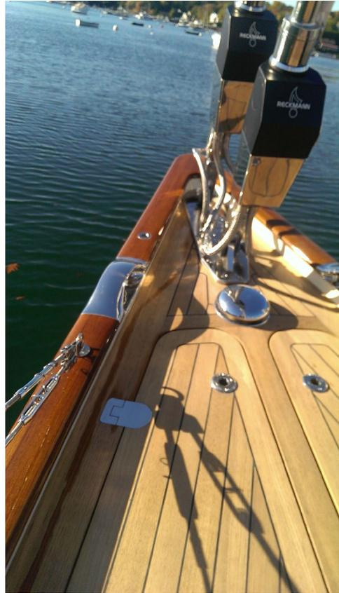
Anchor swing out system to port, chain locker and large storage to stbd. Twin Reckmann furlers forward.
