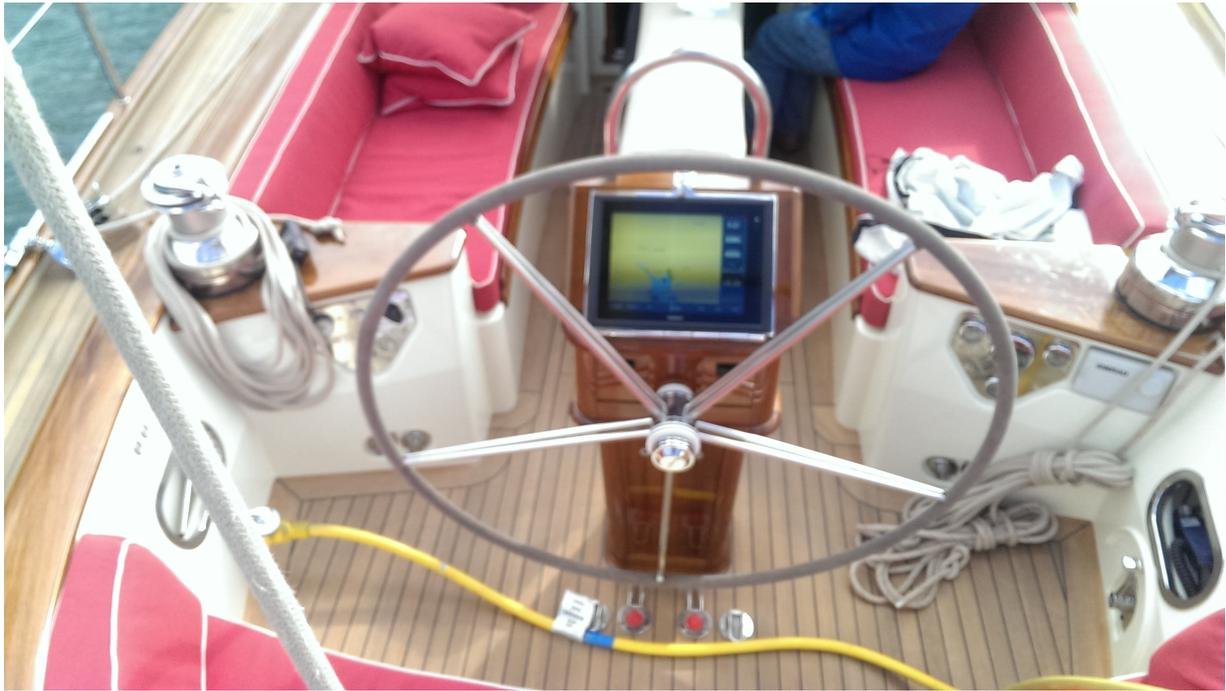
Custom Teak steering pedestal, electric primary winches, thruster controls, mainsheet controls.
